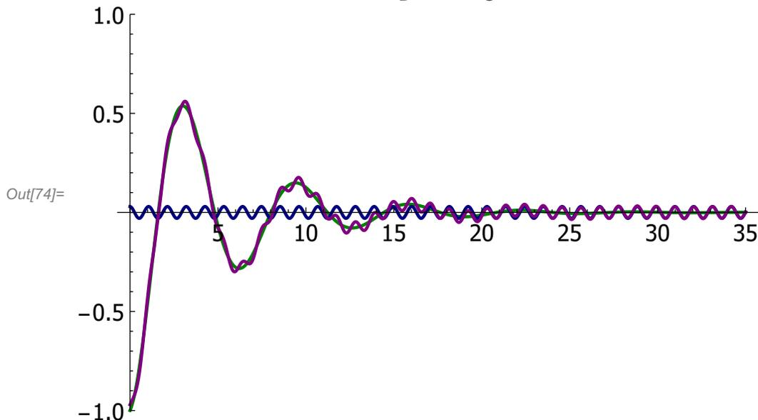
The amplitude of the steady-state term can be seen to increase as  $\omega_D$  approaches the value of  $\omega_S$  then decrease as  $\omega_D$  gets much larger than the value of  $\omega_S$ . This is due to the dependence of the
